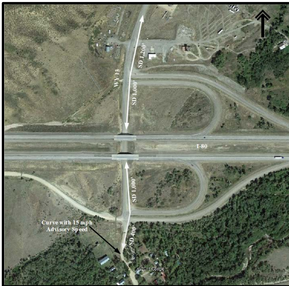
Figure 16. Aerial View I-80/WY 13 Intersection
