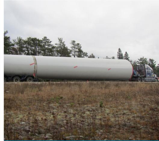
**Equipment Delivery.** Turbine components including the tower, blades and nacelle are delivered to site.
